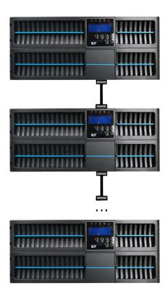
This functionality allows the UPS to work in redundancy, when the power required is less than the nominal power of the single UPS (n + 1), and the power parallel operation (2n) when, for peak current or greater power required, it exceeds the power of the single UPS. This operating selectivity is automatic and instantaneous. Up to 4 units can be connected in parallel, and are available as external manual by-pass accessories for parallel distribution up to 200A (40kVA).
